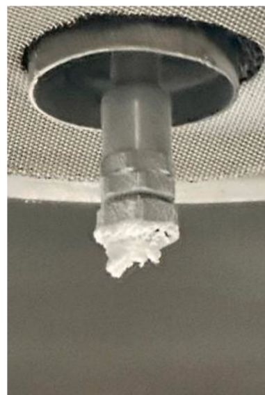
Fig. 5. Deposition on top of the nozzle during the process.
